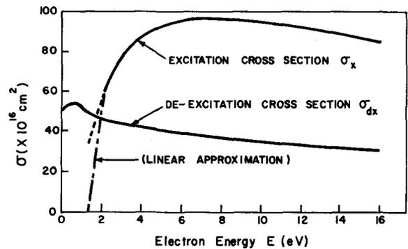
FIG. 1. The  $6s-6p$  excitation and de-excitation electron collision cross sections of cesium calculated by means of the impact parameter method.
