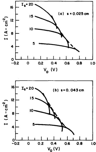
FIG. 7. Calculated thermionic converter performance characteristics for  $T_E = 1785^\circ\text{K}$ ,  $N_0 = 2 \times 10^{16} \text{ cm}^{-3}$ , and  $\phi_e = 1.6 \text{ V}$ .
