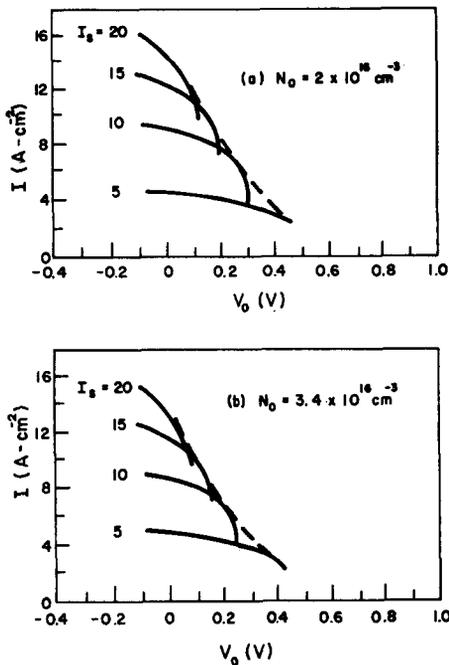
FIG. 6. Calculated thermionic converter performance characteristics for  $T_E = 1608^\circ\text{K}$ ,  $s = 0.025 \text{ cm}$ , and  $\phi_e = 1.6 \text{ V}$ .
