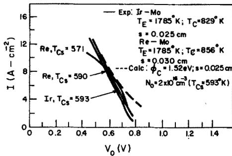
FIG. 10. Comparison of experimental thermionic converter performance characteristics with calculated envelope of optimum performance.
