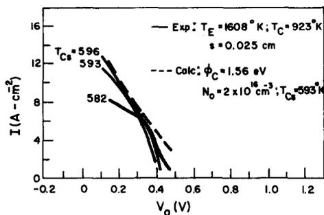
FIG. 8. Comparison of experimental performance characteristics with calculated envelope of optimum performance for a Ta-Mo thermionic converter.
