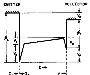
FIG. 5. Schematic of the potential distribution in a thermionic converter.
