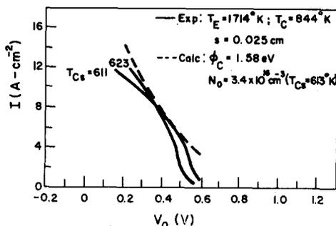
FIG. 9. Comparison of experimental performance characteristics with calculated envelope of optimum performance for a Ta-Mo thermionic converter.
