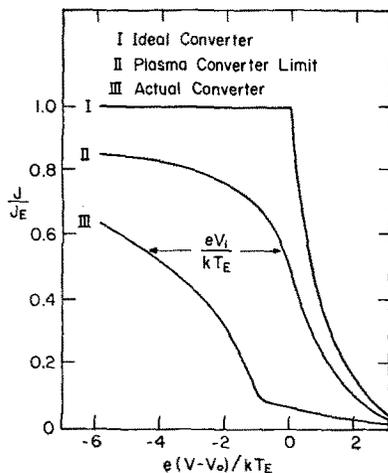
FIG. 2. Comparison of output-current characteristics for different operating conditions.
