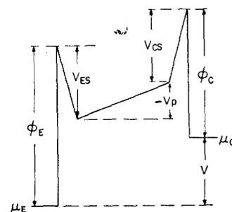
FIG. 1. Motive diagram for thermionic converters operating in the ignited mode.
