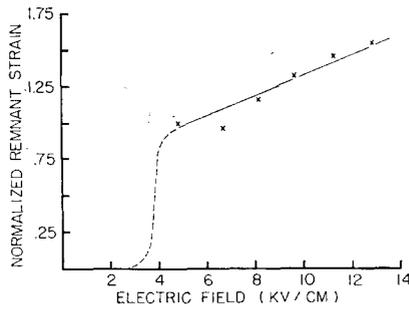
FIG. 4. Normalized strain as a function of applied electric field which clearly shows the existence of a threshold field.
