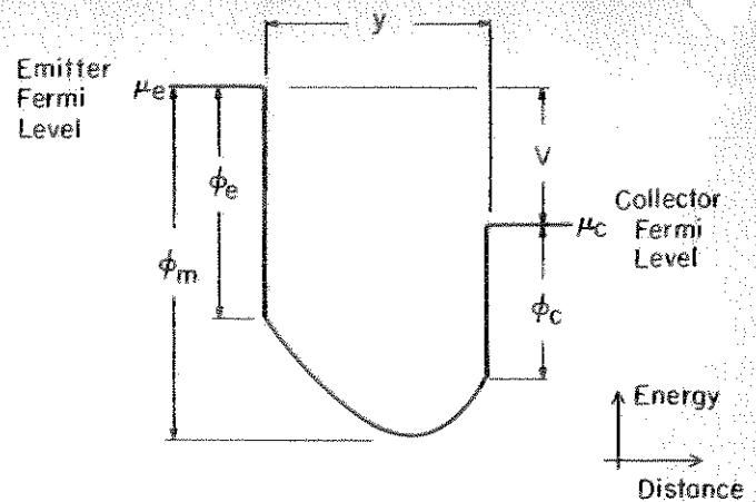
Fig. 2. Potential distribution in a vacuum thermionic converter
