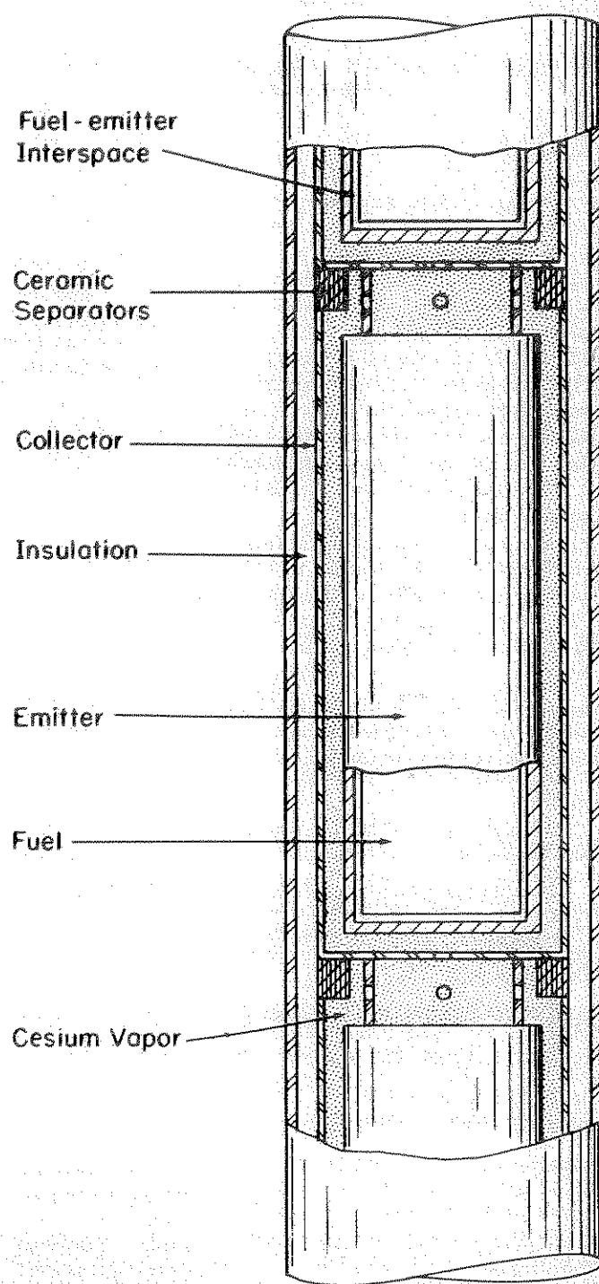
Fig. 16. Schematic of converter integrated into fuel element
