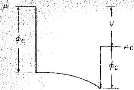
Fig. 3. Unstable potential distribution in a cesium thermionic converter
