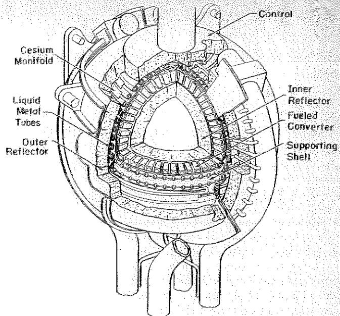
Fig. 14 (right). Schematic of thermionic nuclear reactor cooled by means of liquid metal loop
