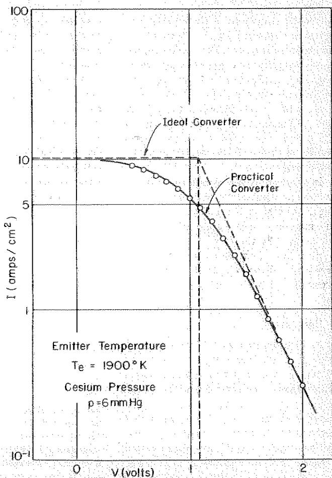
Fig. 5. Typical current-voltage characteristics of ideal and practical converters
