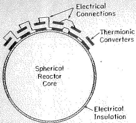
Fig. 11. Schematic of thermionic nuclear reactor with converters attached to outer surface of reactor core
