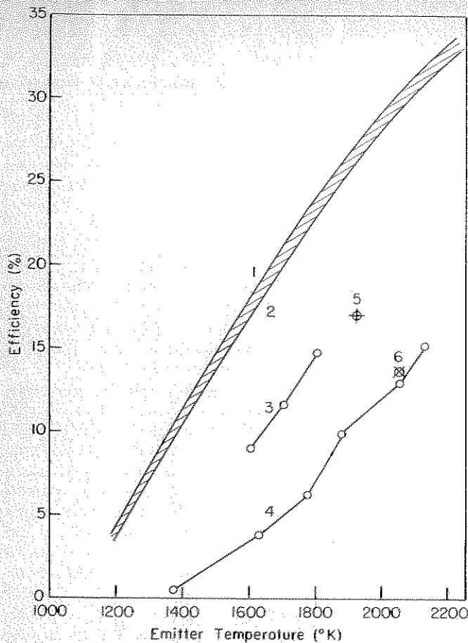
Fig. 6. Thermal efficiency of thermionic converters
