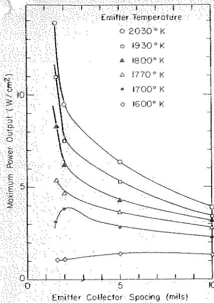
Fig. 8. Optimum electric power density as a function of interelectrode spacing and emitter temperature
