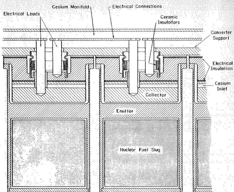
Fig. 12. Schematic of converter fuel-slug units
