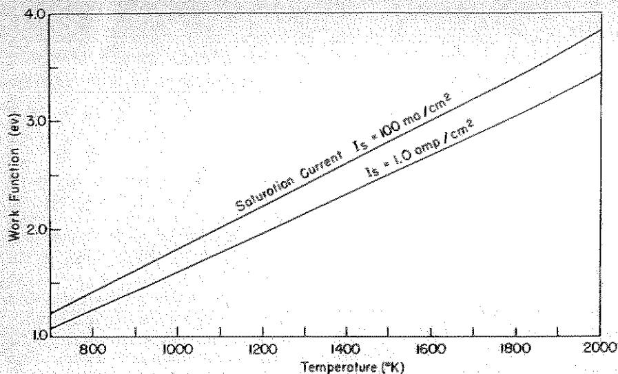
Fig. 9. Collector work-function versus collector temperature for negligible back-emission
