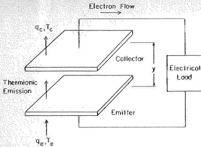
Fig. 1. Schematic of thermionic converter
