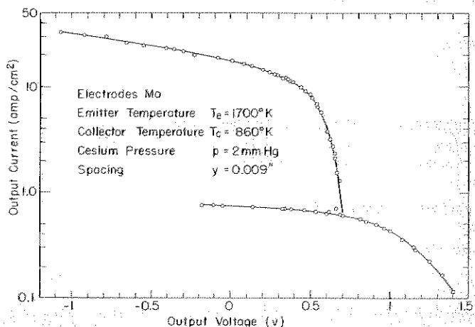
Fig. 7. Extinguished and ignited mode current-voltage characteristics of a cesium thermionic converter
