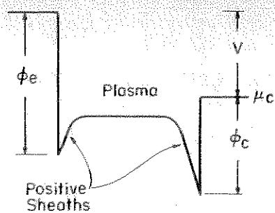
Fig. 4. Potential distribution in a cesium thermionic converter with an ion current greater than 1/500 of electron current
