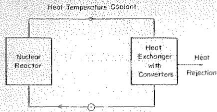
Fig. 10. Schematic of thermionic nuclear reactor with converters separate from the reactor core
