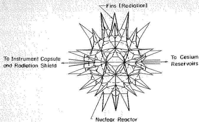
Fig. 13 (left). Schematic of thermionic nuclear reactor radiating into free space
