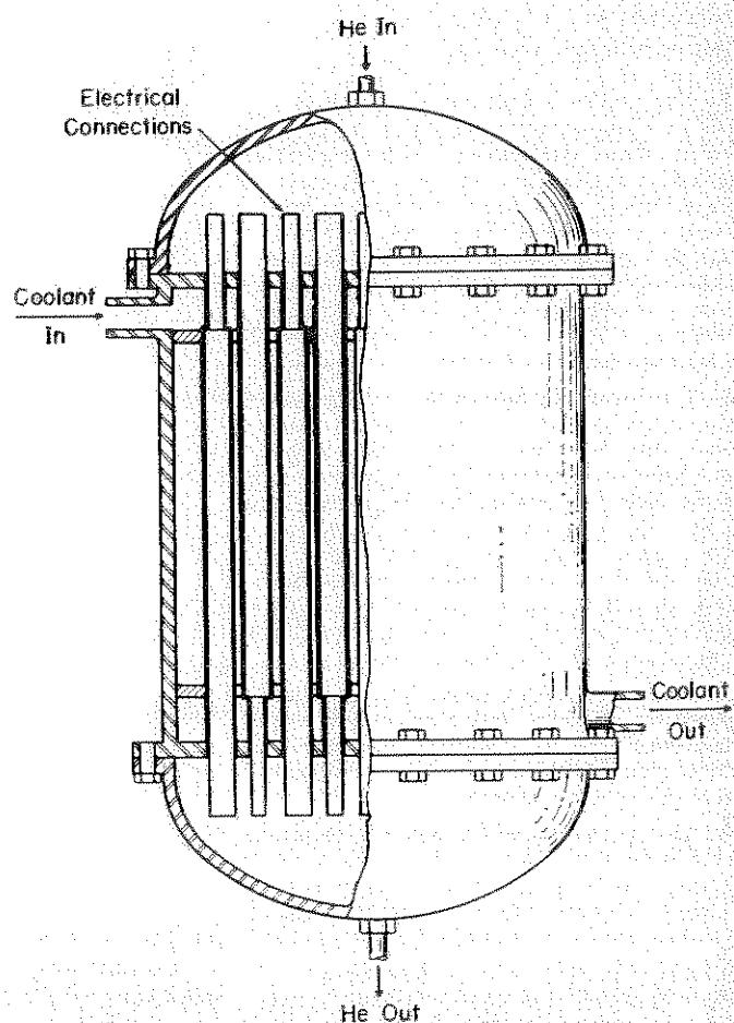
Fig. 15. Schematic of thermionic nuclear reactor with converters integrated into fuel elements
