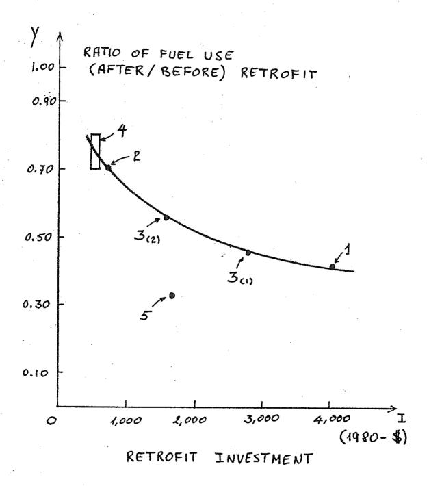
Figure 2 Ratio of Fuel Use -- After/Before -- Retrofit versus Retrofit Investment
